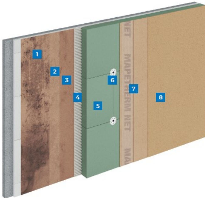
Mapetherm X2 System: doubling of the insulation system with a reinforced cycle
